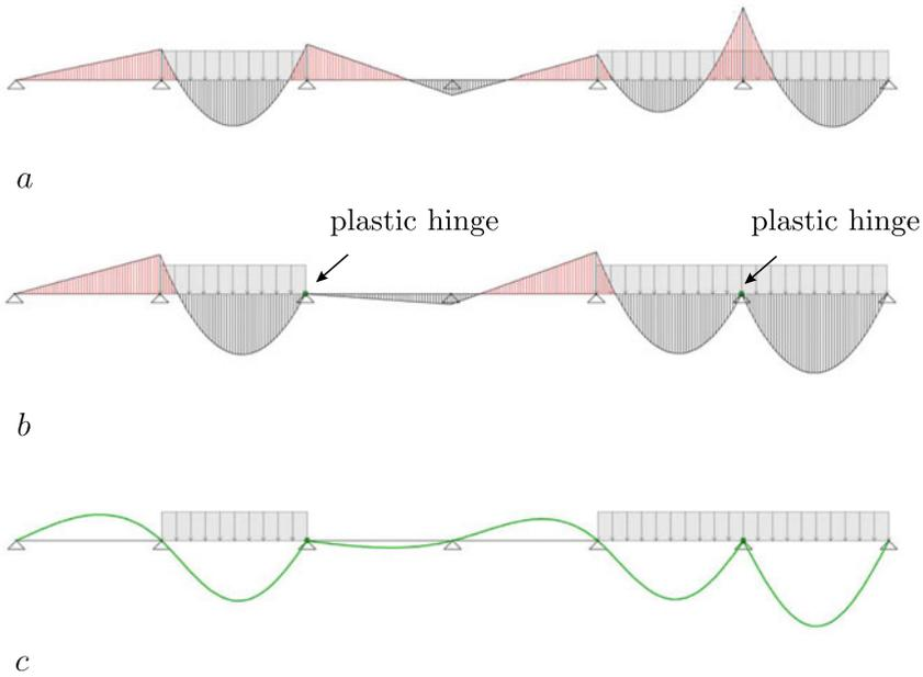
**Fig. 5.34** Adding plastic hinges to a continuous beam, **a** original moment distribution, **b** after the hinges have been added, **c** deflection
