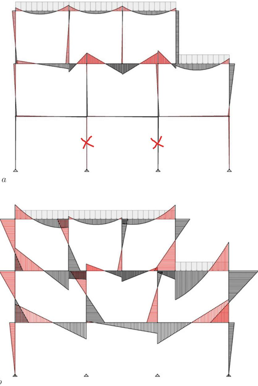
**Fig. 5.32** One-click reanalysis (without modification of the stiffness matrix), **a** the crossed-out elements, **b** moment distribution without the two columns
