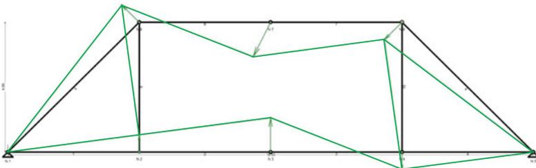
Fig. 5.33 Possible infinitesimal motions in a frame can be discovered with the “twofold” Gauss
